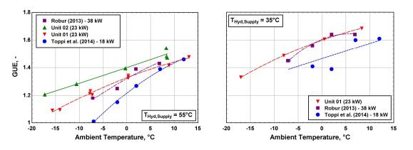
Figure 7: GUE comparison at 55 and 35°C hydronic supply temperatures
