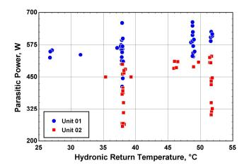
Figure 6: Parasitic power as a function of hydronic return temperature
